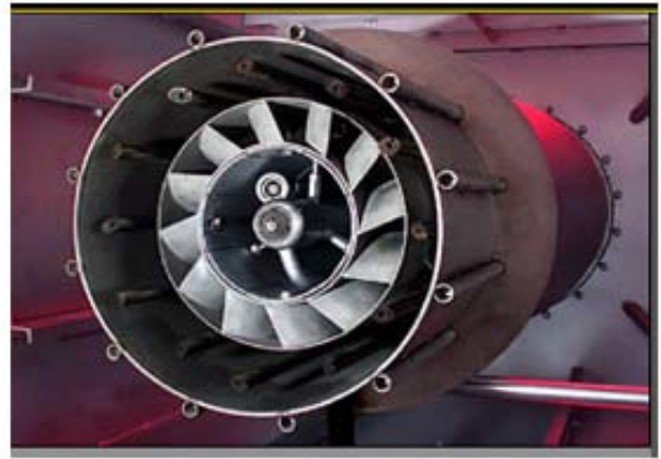
Fig. 2. Industrial Fuel/Air Swirler (Courtesy of National Combustion Equipment, Inc.)
